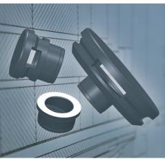
The FLUXX® Degassing Inserts make it possible for gaseous substances to diffuse, thereby preventing pressure from building up and decreasing in the containers. The membranes are hydrophobic as well as oleophobic, and as a result they are not moistened even by liquids with a low surface tension and remain fully breathable at all times.
